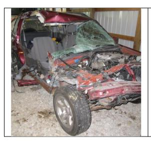
There was extensive front-end and passenger side damage to the Suzuki. The hood and front fender were torn from the vehicle. The flatbed of the tow truck cut through the windshield and the A-Pillar. The passenger side front and rear doors were removed from the vehicle as a result of the flatbed of the truck cutting through the vehicle.
